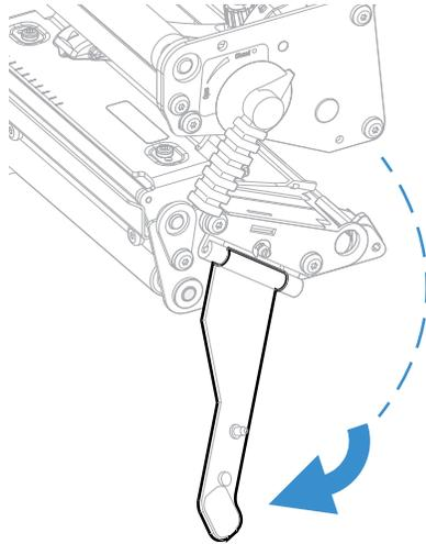
4. Turn the printhead lift lever counter-clockwise to raise the printhead.
