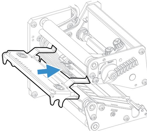
11. Turn the printhead lift lever clockwise so the magnet engages the printhead bracket.
