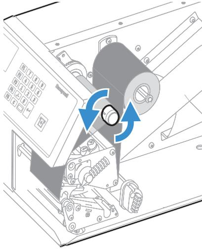
11. Turn the printhead lift lever clockwise to lower the printhead.
