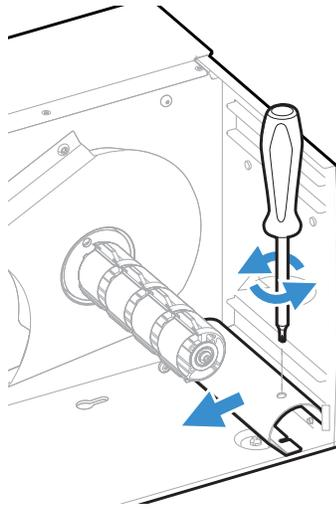
6. Remove the tear bar from the print unit and replace it with the guide plate.
