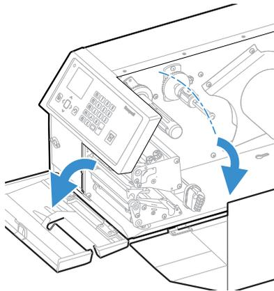
3. Turn the printhead lift lever counter-clockwise to raise the printhead.
