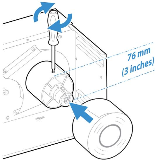
7. Fit a new roll of media on the supply post and push the roll in as far as it will go.
