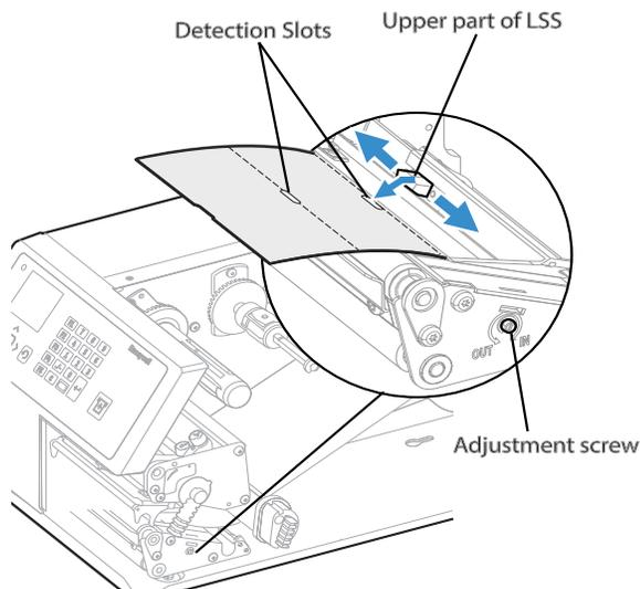
2. Look at the print mechanism from the front with the printhead lifted to make sure that the point of detection on the upper sensor is aligned with the center of the slots or marks in the media.
