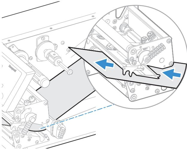
11. Pull out approximately 40 cm (15 in) of labels and remove the labels from the liner.
