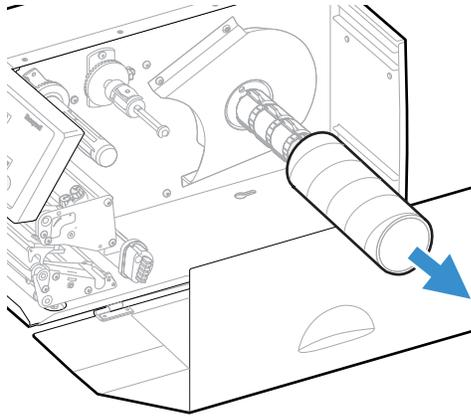
6. If you are using a media roll with a 76 mm (3 in) core, fit an adapter on the media supply hub.
