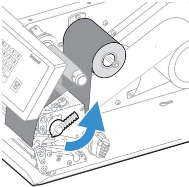
4. Remove any empty core from the media supply hub.
