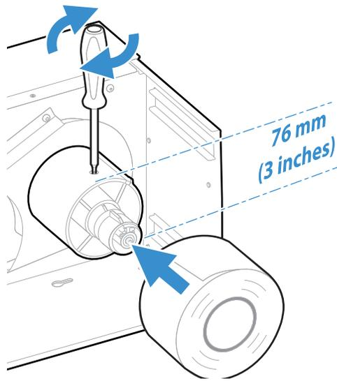
8. Fit a new roll of media onto the media supply hub and push the roll in as far as it will go.
