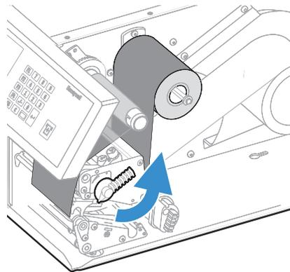
5. Remove any empty core from the media supply hub.
