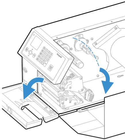
3. Turn the printhead lift lever counter-clockwise to raise the printhead.
