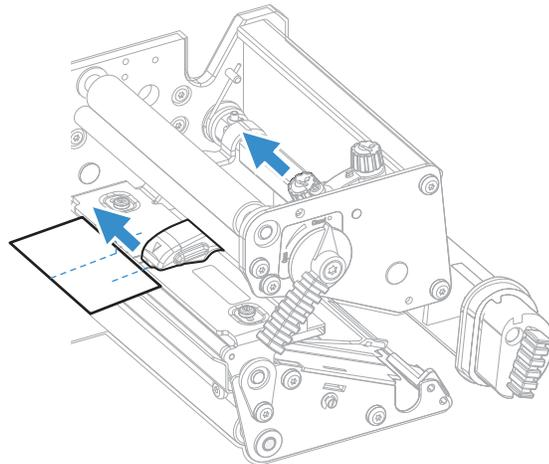
6. When the pressure arm is centered, tighten the knob to secure the arm. **Do not over-tighten the knob.**
