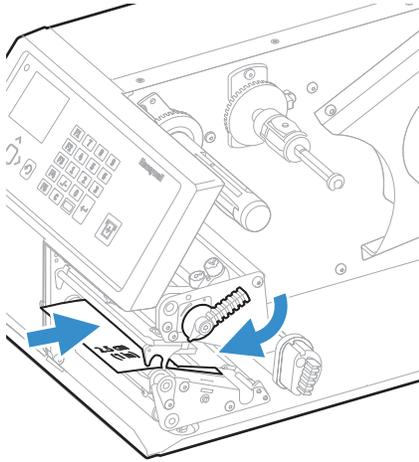
7. Pull out the cleaning card and raise the printhead.
