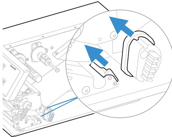
13. Route the media through the cutter between the two guide plates.
