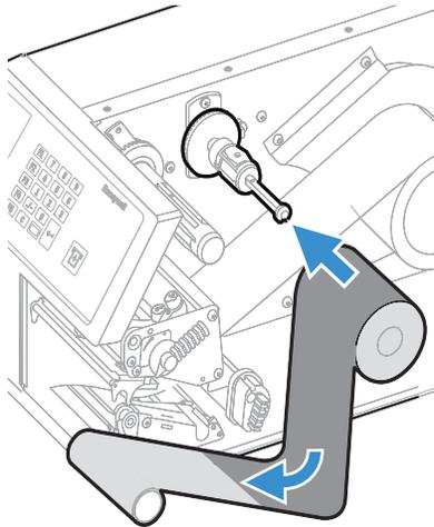
7. Without releasing the ribbon, turn the printhead lift lever clockwise to lower the printhead and lock the ribbon.
