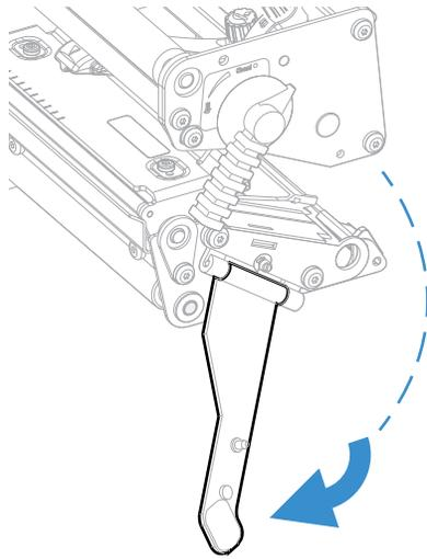
3. Turn the printhead lift lever counter-clockwise to raise the printhead.
