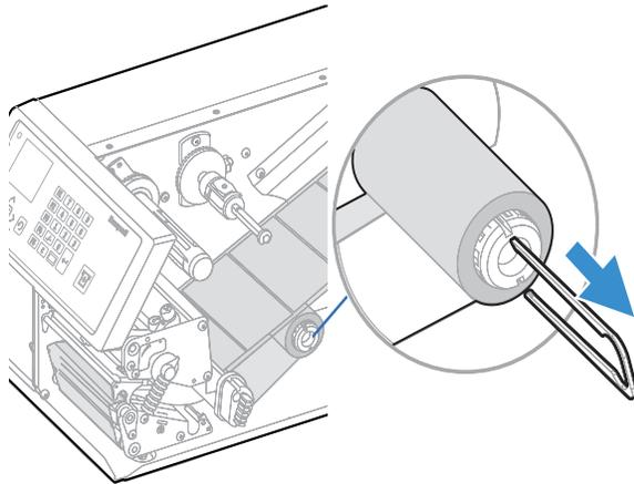
6. Remove any empty core from the media supply hub.
