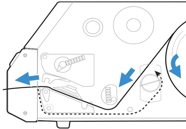
10. Lower the printhead by turning the printhead lift lever clockwise.
