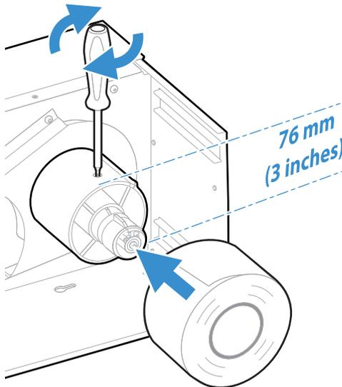
7. Fit a new roll of media onto the media supply hub and push the roll in as far as it will go.
