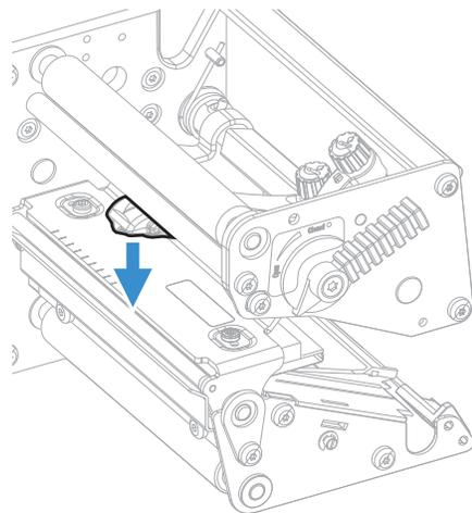
7. Disconnect the hooks of the printhead bracket from the shaft and pull out the printhead as far as the cables allow.
