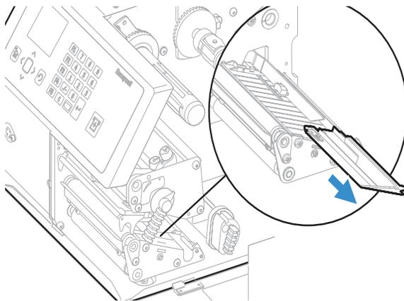
3. Clean the guides with a cleaning card or soft cloth moistened with isopropyl alcohol. Be careful not to scratch the guides.
