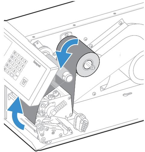
9. Turn the printhead lift lever counter-clockwise to raise the printhead.
