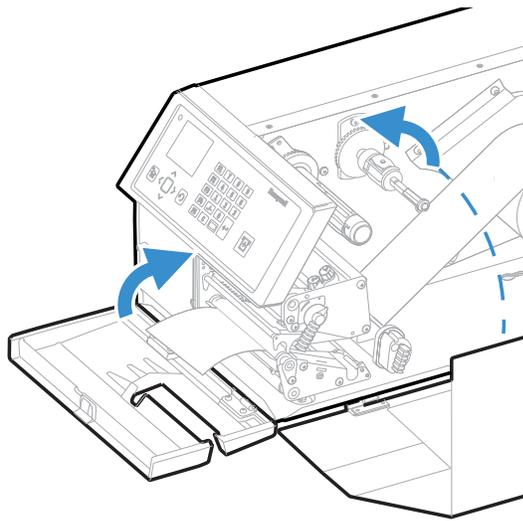
18. Press the **Print/Feed** button to advance the media and adjust the media feed.
