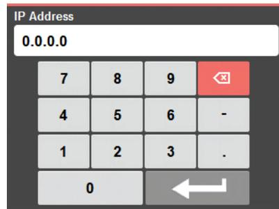
To access the extended numeric keypad, select the 123 key on the alphanumeric keypad.
