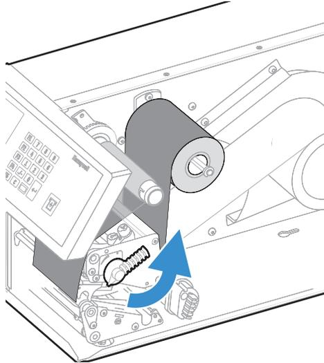
5. Pull out the red clip on the liner take-up hub and dispose of any wound-up liner.
