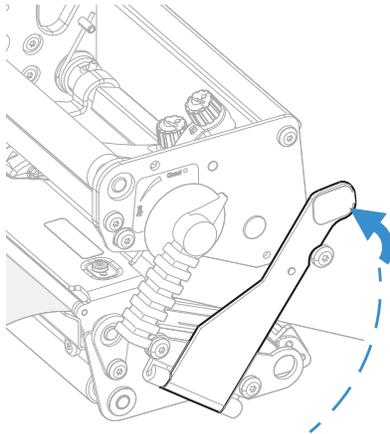
16. Adjust the position of the red edge guides so that the media is guided with a minimum of play.
