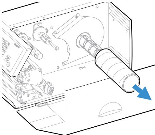
7. If you are using a media roll with a 76 mm (3 in) core, fit an adapter on the media supply hub.
