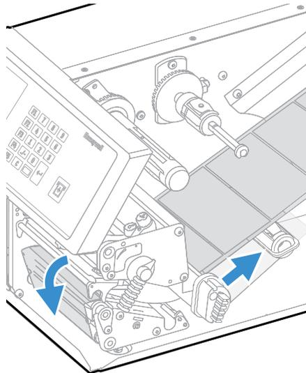
13. Secure the liner to the take-up hub with the red clip and rotate the hub until the media is pulled tight.
